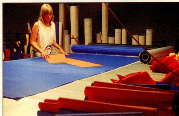
Engineering manager Tom Price (above) calls up engineering specs from Quicksilver's database. Dacron for the GT-500's wings and tail are cut to size in the sail loft (below).
